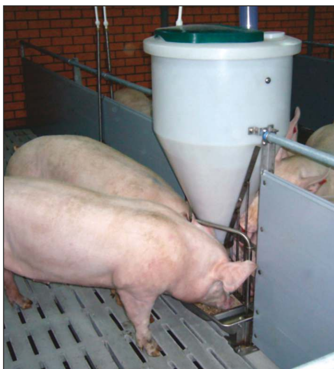
fattening sector: a pen equipped with the single-sided MULTIMAT T automatic feeder
