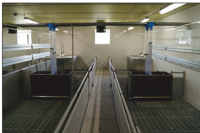
weaner sector: a pen equipped with a double-sided automatic weaner dry automatic feeder for 7 stands on each side.
