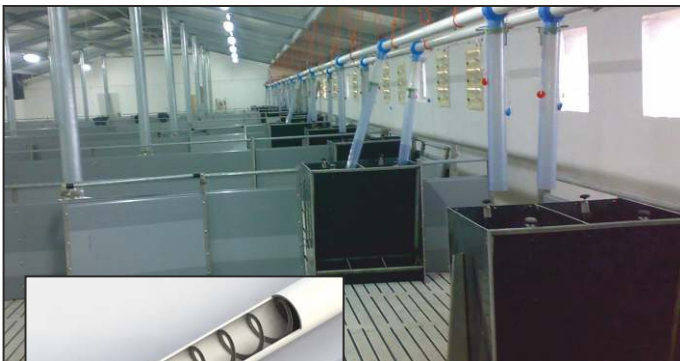
a fattening house equipped with spiral feed distribution system
